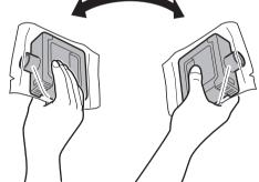
• Failure to shake the ink tanks may result in reduced print quality because ink ingredients have settled on the bottom of the tank.
