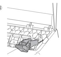
• Make sure the ink tank lock lever stays in the locked position.
