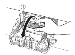
Grasp the grip in the center of the print head locking cover ② and open it. Do not touch the contacts (A) on the carriage.
