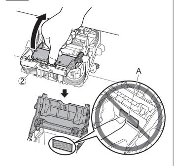
1 Remove the print head from the box and bag, and peel off the fixing tape.
