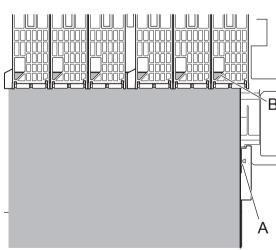
Lower the release lever to lock the paper and close the top cover.
