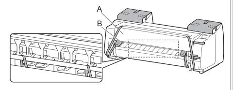
With 3 people holding the carrying handles under the printer on both ends, lift the printer.
